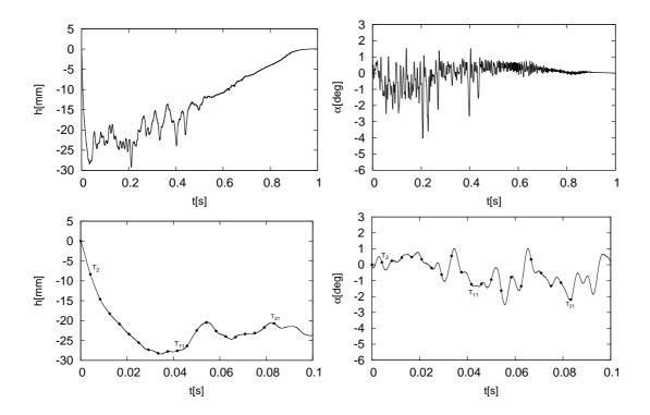
Figure 5: The numerical results for heavy gust. The aeroelastic response of the typical airfoil section for far field velocity  $U_{\infty} = 15 \,\mathrm{m/s}$  and gust velocity  $V_G = 5 \,\mathrm{m/s}$  (top). The detail of the response during the first 0.1 s (bottom).
