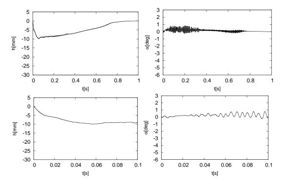
Figure 4: The numerical results for light gust. The aeroelastic response of the typical airfoil section for far field velocity  $U_{\infty} = 15 \,\mathrm{m/s}$  and gust velocity  $V_G = 1.5 \,\mathrm{m/s}$  (top). The detail of the response during the first 0.1 s (bottom).
