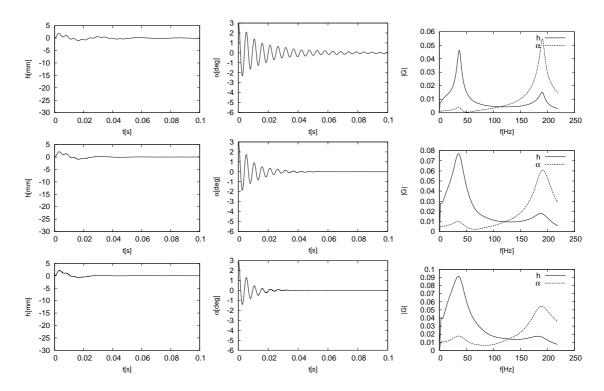
Figure 2: Aeroelastic response and its spectra for the far field velocity  $U_{\infty} = 5 \,\text{m/s}$  (top),  $U_{\infty} = 10 \,\text{m/s}$  (middle) and  $U_{\infty} = 15 \,\text{m/s}$  (bottom).
