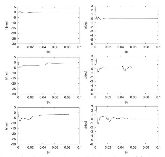
Figure 3: Aeroelastic response for the far field velocity  $U_{\infty} = 30 \,\text{m/s}$  (top),  $U_{\infty} = 50 \,\text{m/s}$  (middle) and  $U_{\infty} = 60 \,\text{m/s}$  (bottom).
