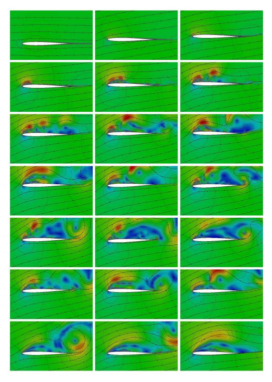
Figure 6: The flow pattern at the equidistant time instants  $T_k=k\Delta T$  marked in Fig. 5,  $\Delta T=2\times 10^{-4}\,\mathrm{s}.$
